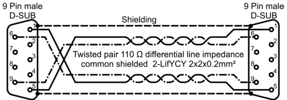
Figure 1: Electrical connection SL2-100
