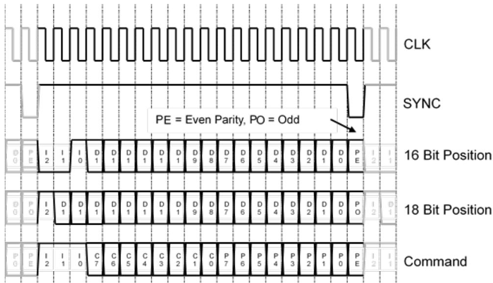
Figure 3: XY2-100-E Command Channel Frame Types
