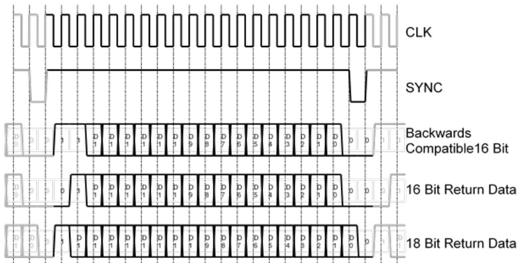
Figure 4: XY2-100-E Return Channel Frame Types
