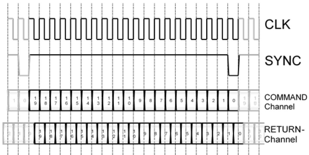
Figure 2: XY2-100-E Frame Timing
