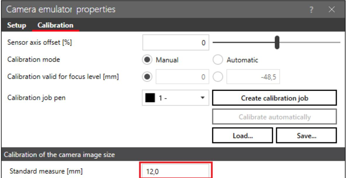
The screenshot shows the 'Camera emulator properties' dialog box with the 'Calibration' tab selected. The 'Standard measure [mm]' field is highlighted with a red box and contains the value '12,0'. Other fields include 'Sensor axis offset [%]' (0), 'Calibration mode' (Manual selected), 'Calibration valid for focus level [mm]' (0), and 'Calibration job pen' (1 -). Buttons for 'Create calibration job', 'Calibrate automatically', 'Load...', and 'Save...' are also visible.
